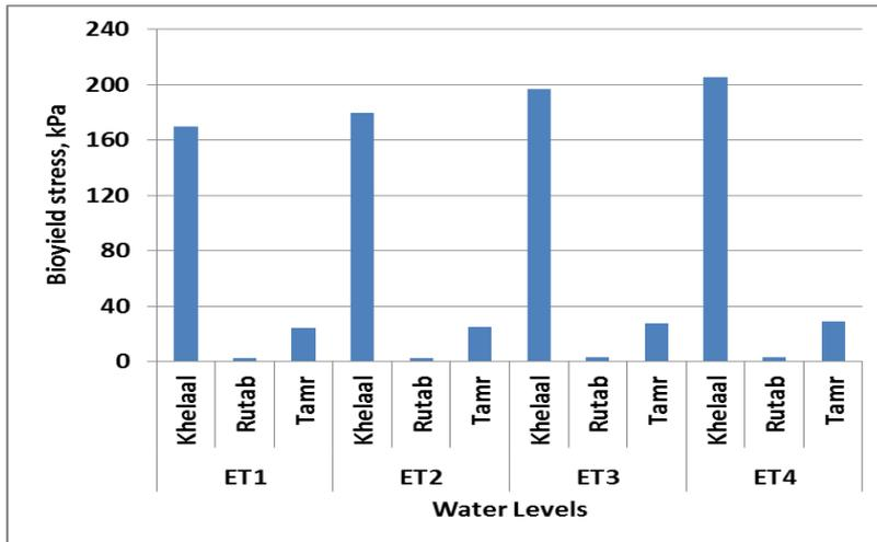
**Fig. 7.** Bio-yield stress for different irrigation water levels at different ripening stages of date fruit.
