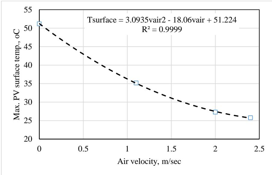
**Fig. 8.** The relationship between air velocity and PV module surface temperature.
