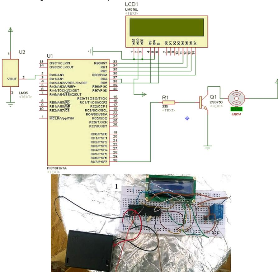
**Fig. 5.** Microcontroller schematic and circuit of temperature control unit
