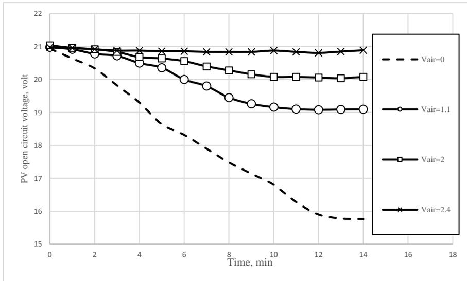
**Fig. 7.** Effect of air velocity on PV module open circuit voltage.
