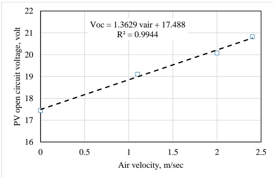
**Fig. 9** The relationship between air velocity, PV open circuit voltage.
