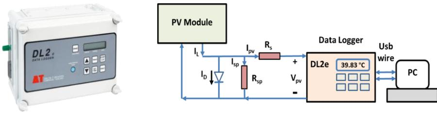
**Fig. 4.** Schematic diagram shows the connection of data logger with computer and PV modules (Rashwan M. A.; Jailany A. T. et al., 2015)
