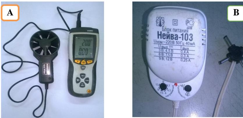
**Fig. 3.** (A) Thermo anemometer **VA893**, (B) DC voltage adapter **NEVA-103**.
