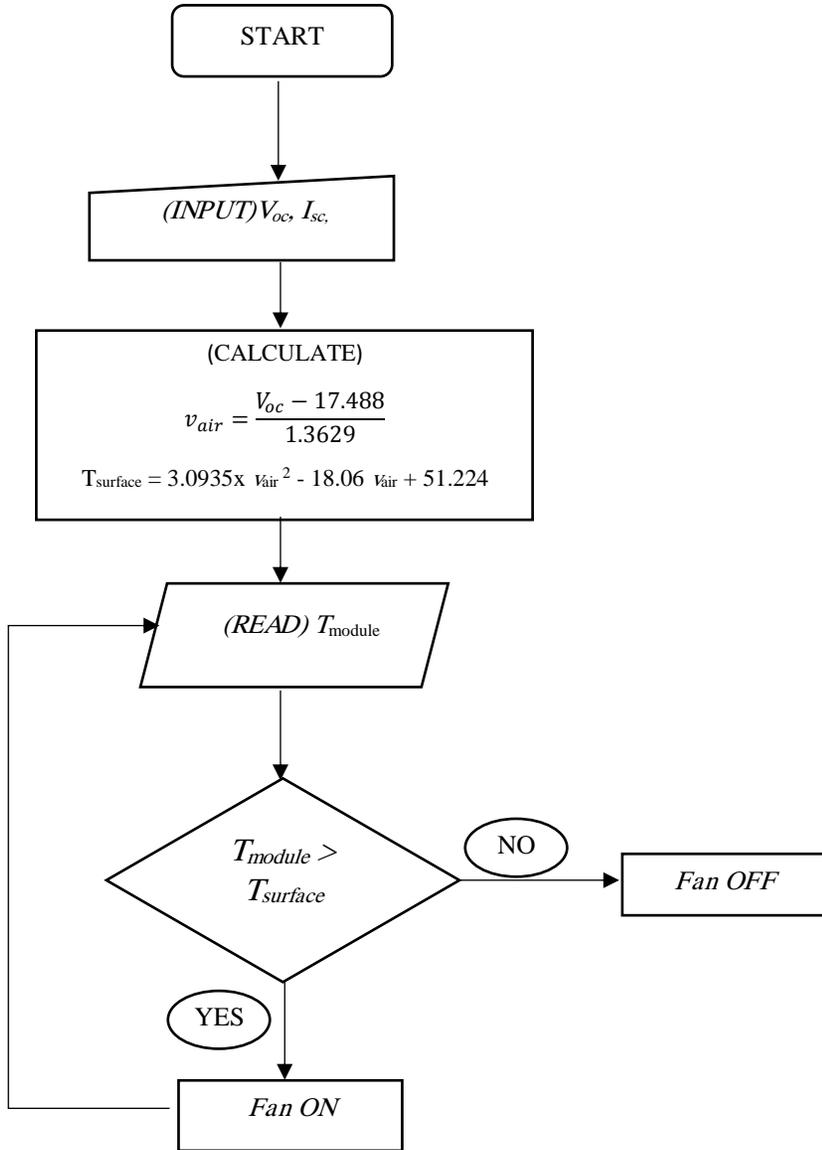
**Fig. 10.** Microcontroller programming flow chart
