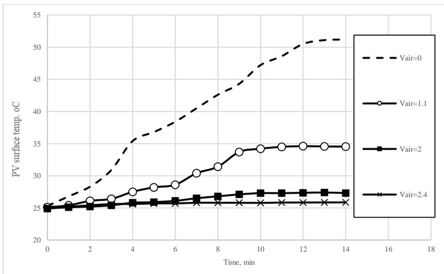
**Fig. 6.** Effect of air velocity on PV module surface temperature
