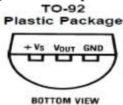
**Figure 3.** Connection diagram of temperatures sensor of LM35
