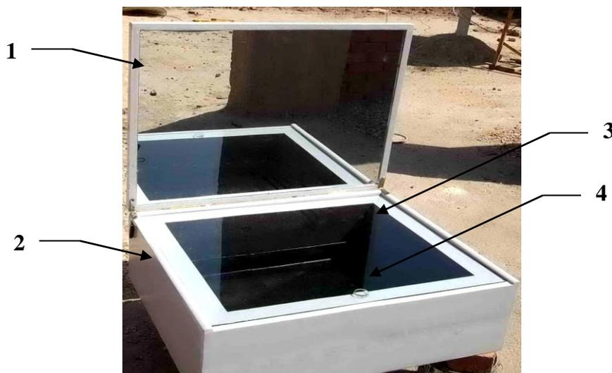
1. Mirror reflector 2. Cooker frame 3. Glass cover 4. Absorber plate
