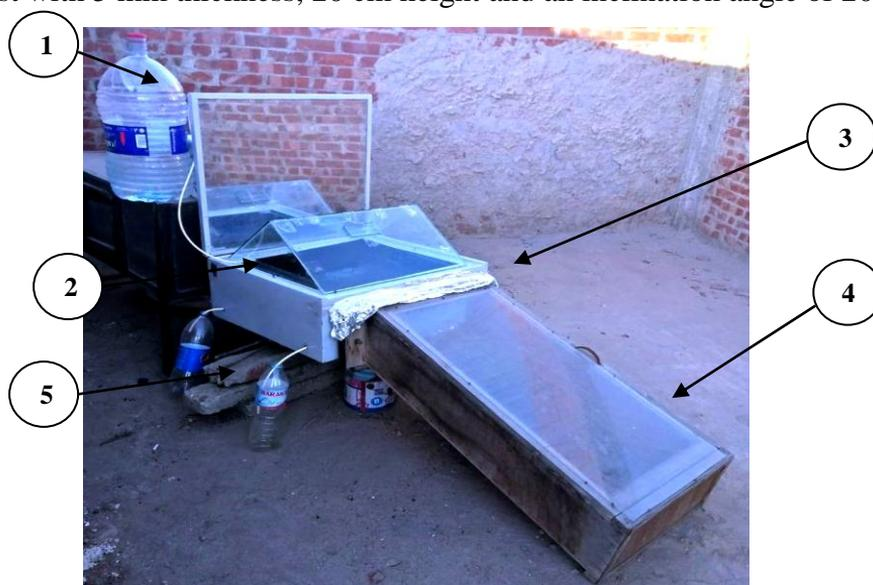
1. Saline water tank      2. Feeding inlet      3. Box type cooker
