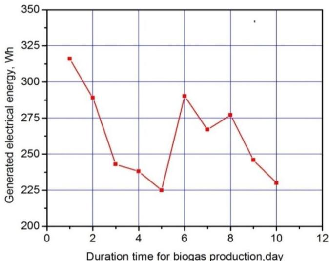
Figure 4: The electrical energy produced from biogas during the operating of electrical generator at full throttle fuel position.
