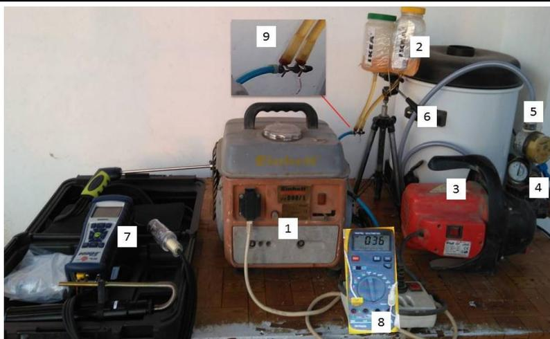
1-Einhell800S two stroke SI. Generator 2-Two external tank for bioethanol and Gasoline fuels 3- Water pump as load 4-Pressure gauge manometer 5-Flow meter 6- Water tank 20 7-Bachrach gas analyzer 8-Multimeter MR445 9-Three way valves to obtain the blend fuel ratios
