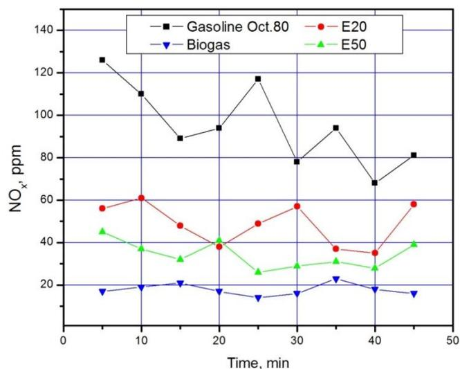
Figure 8: Concentration of NO<sub>x</sub> produced from different biofuels during the operating of electrical generator at full throttle fuel position.
