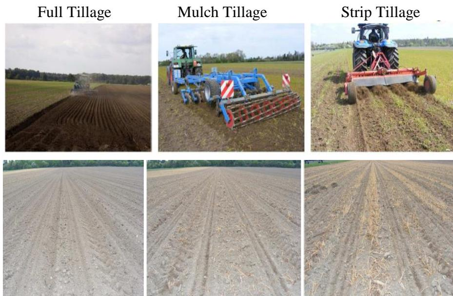
Fig 2: Soil tillage treatments (Full tillage, mulch tillage and strip tillage).
