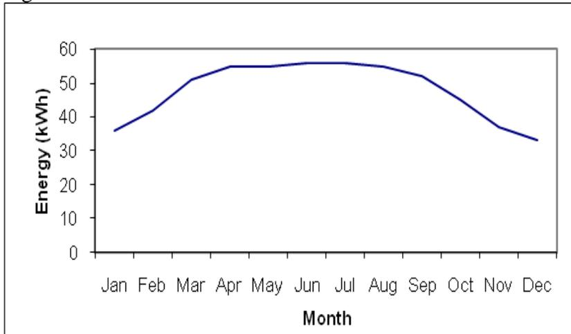
**Fig. (2):** Average daily energy (kWh) produced by the solar – powered pumping system used throughout the year
