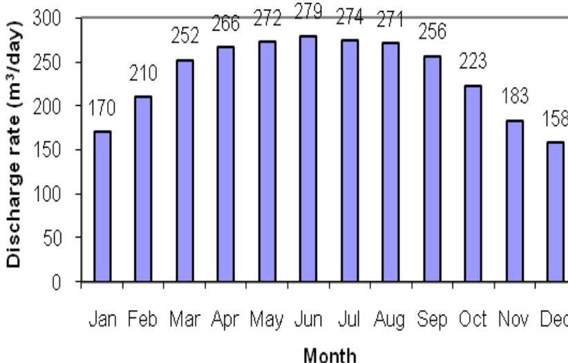
**Fig. (3):** Average daily discharge rate (m<sup>3</sup> day<sup>-1</sup>) of the solar – powered pumping system used over the year
