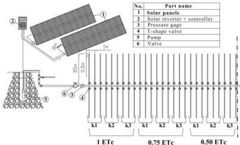
**Fig. (1):** A schematic diagram showing the solar – powered system connected with the drip irrigation network; ETe –crop water requirements and  $k_1$ ,  $k_2$ ,  $k_3$  – potassium fertilization rates
