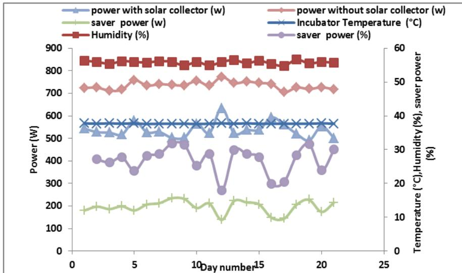
Fig (8): The incubator data in the experimental period from 7<sup>th</sup> to 28<sup>th</sup> February 2017
