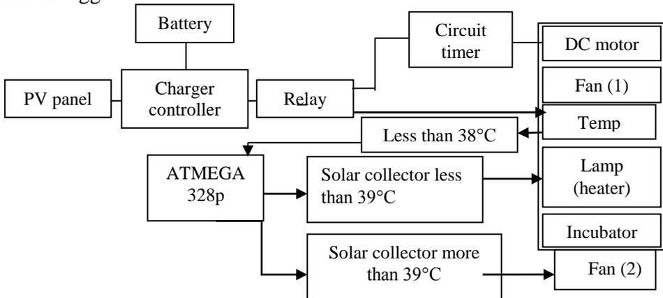
Fig (1): Block diagram of the incubator solar energy
