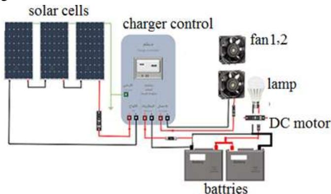
Fig (6): The Solar Energy Components.
