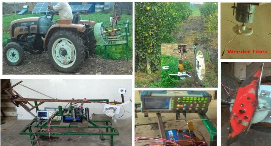
Fig.4: The manufactured swing mechanical arm with electric weeder in laboratory and field conditions.
