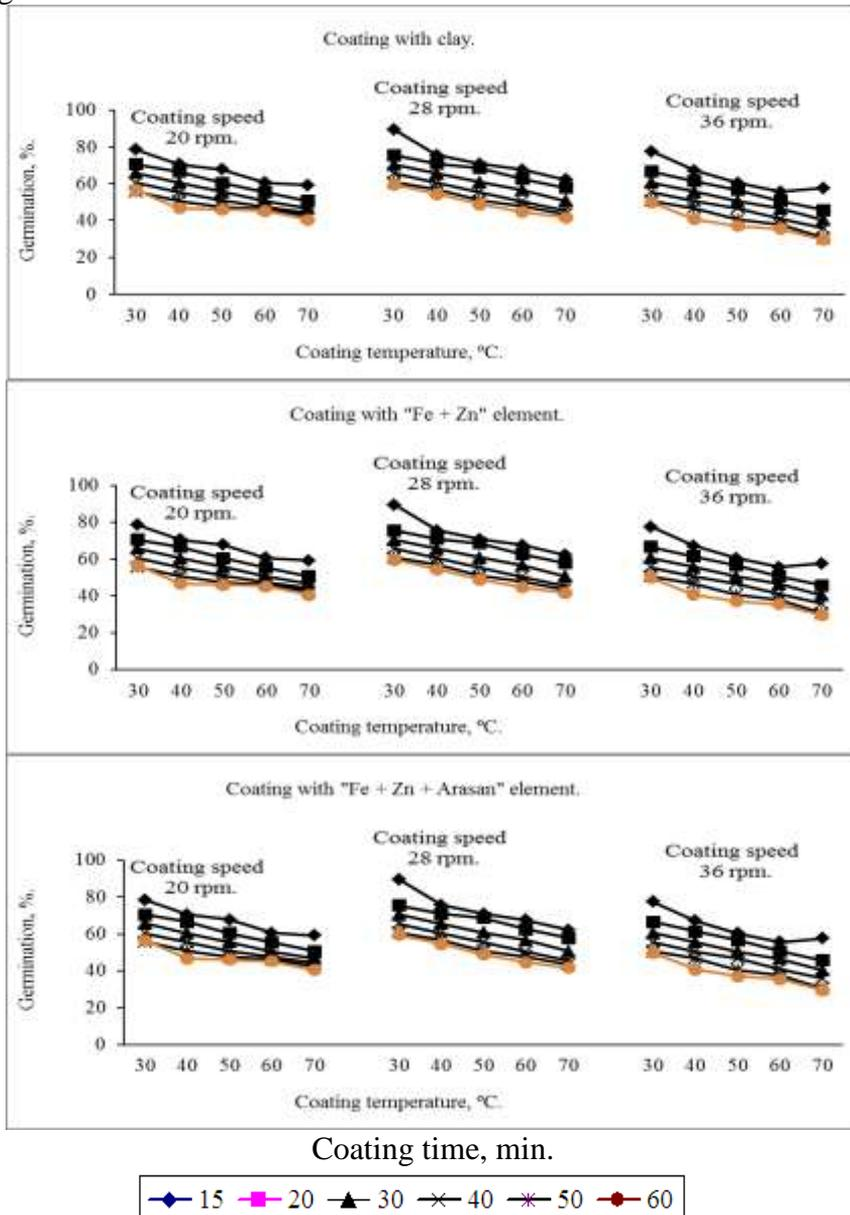
Fig. 5: Effect of coating temperature and time, by “Fe + Zn”, “Fe + Zn + Arsan” and clay on the maize seeds germination and at constant seed batch mass of 2.5 kg.
