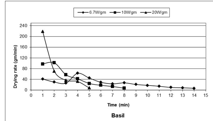
Figure (2) Effect of drying time on the behavior of drying rate according to different microwave power densities
