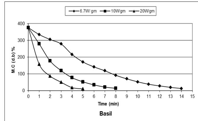
Figure (1) Moisture content versus drying time according to different microwave power densities.
