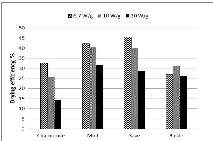
Figure (4) Influence of microwave power density on drying efficiency.
