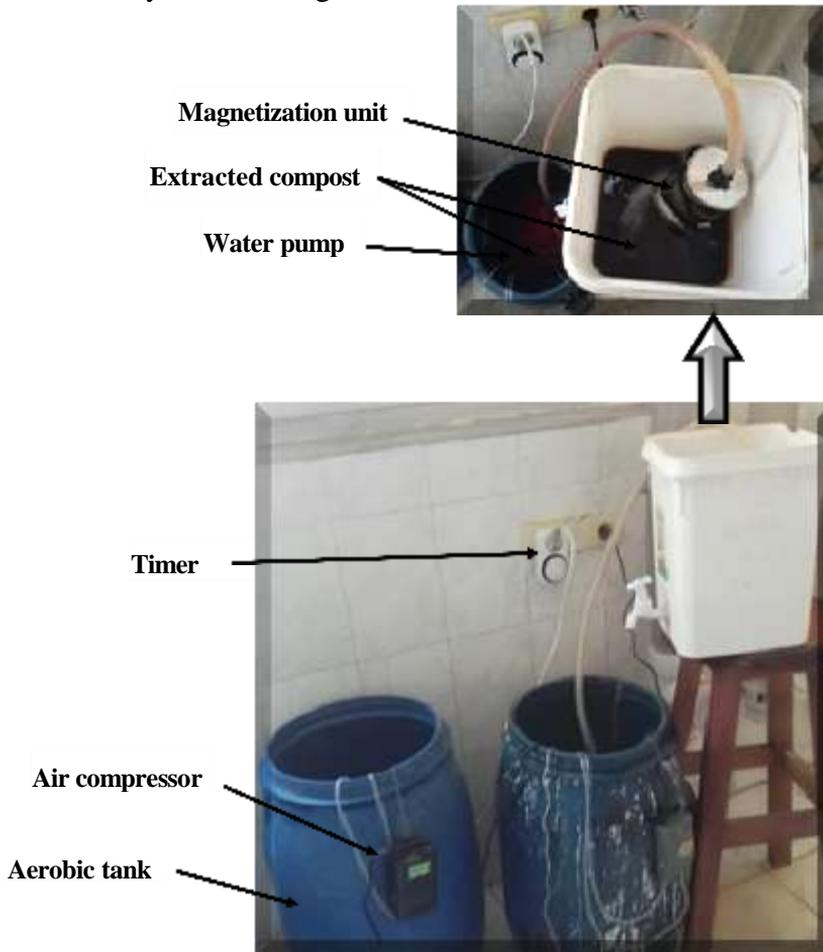
**Fig. 1: The compost extraction system.**
