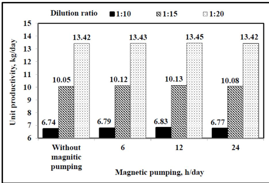
**Fig. 2:Effect of magnetic pumping on system productivity.**
