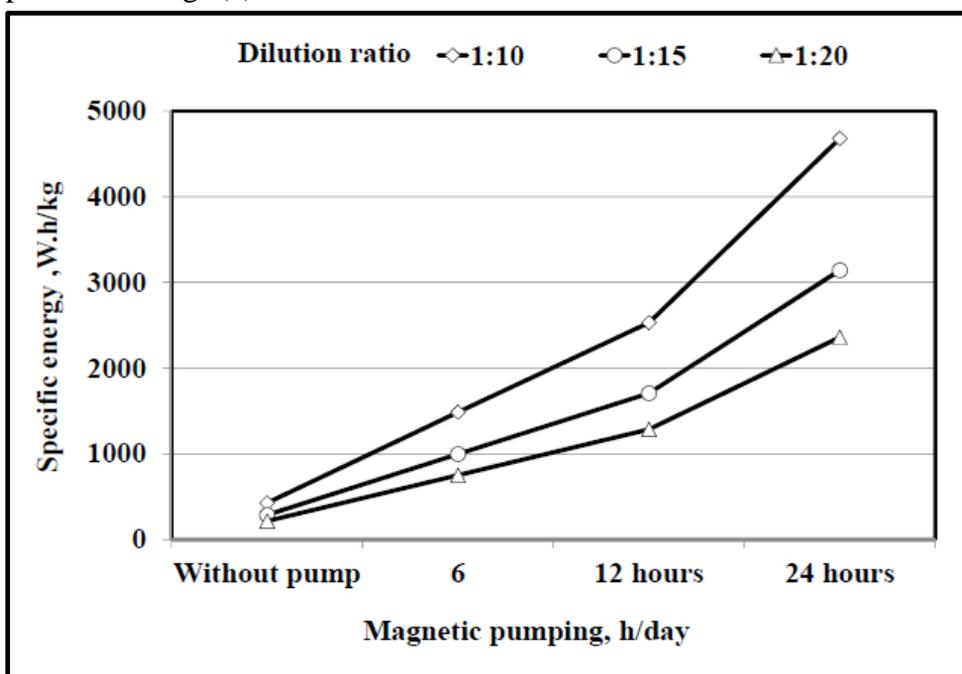
**Fig. 4: Effect of magnetic pumping on energy requirements.**
